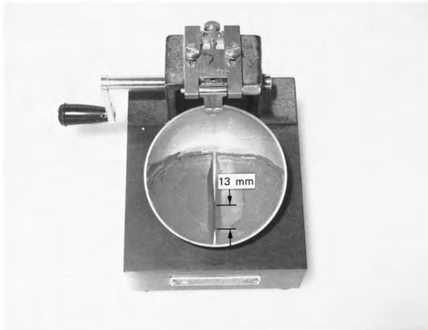
FIG. 8 Soil Pat After Groove Has Closed
