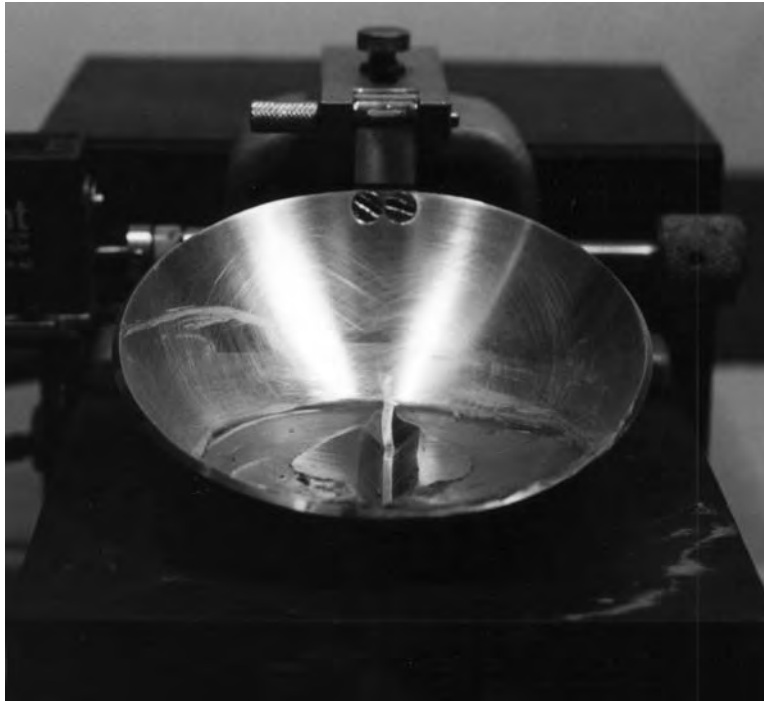
FIG. 7 Grooved Soil Pat in Liquid Limit Device
