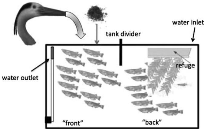
FIGURE 1. Configuration of each aquarium used in experiments with Japanese medakas. The simulated predation treatment involved the presence of a great blue heron decoy (see Methods).
