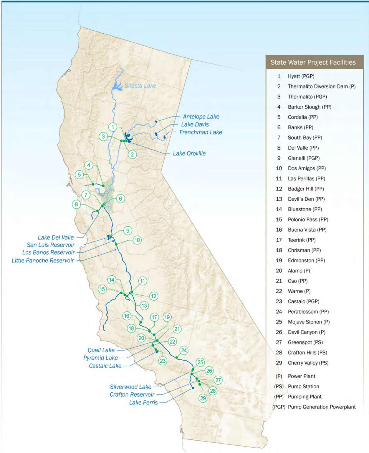
Figure 2-1. Primary State Water Project Facilities
