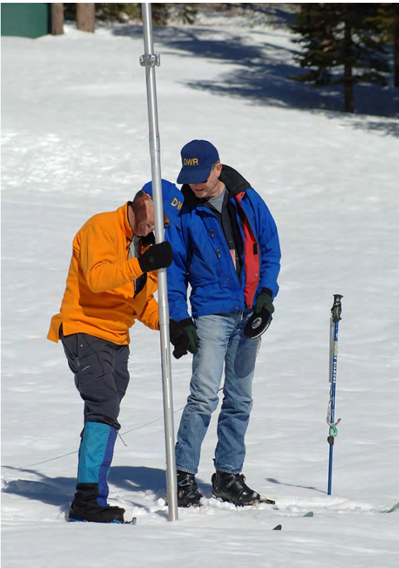
DWR measures the water content of snowpack in the northern Sierra Nevada to forecast snowmelt runoff.
